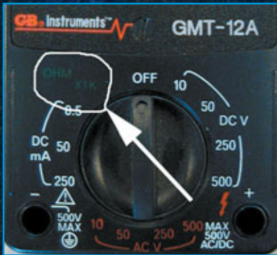
4. The third most common function is for measuring resistance.
